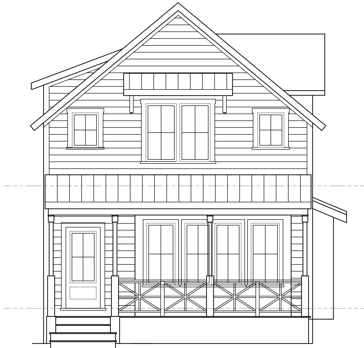
EAST ELEVATION SCALE: 1/4" = 1'-0"
