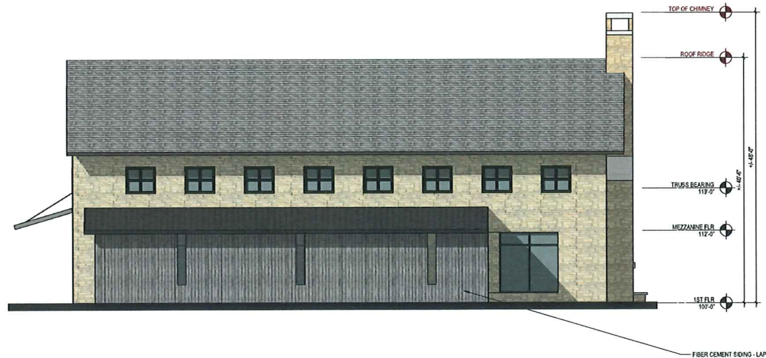
D2 RETAIL BLDG 1 NORTH ELEVATION 1/8" = 1'-0"
