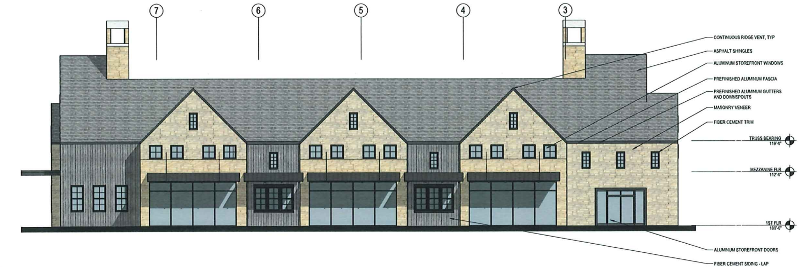
B1 RETAIL BLDG 2 WEST ELEVATION 1/8" = 1'-0"
