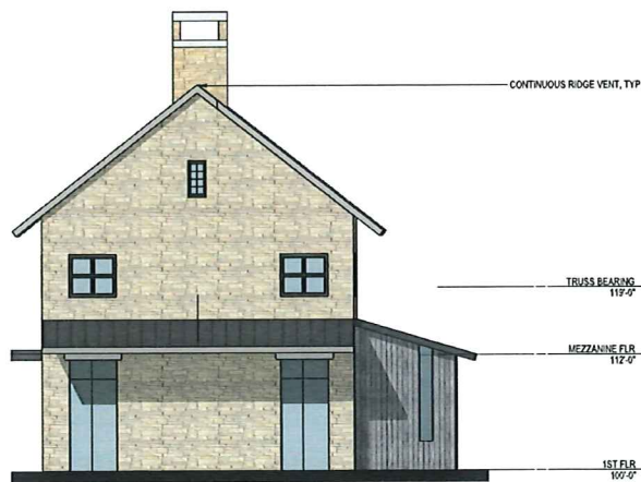
A1 RETAIL BLDG 1 EAST ELEVATION 1/8" = 1'-0"
