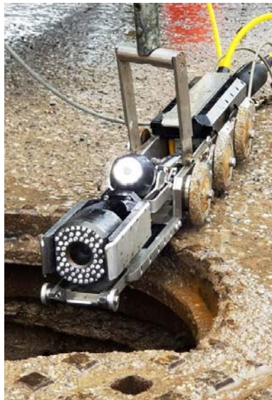
Figure 1 - CTV Mounted Robot Crawler (image from multiVIEW Locates Inc.)
